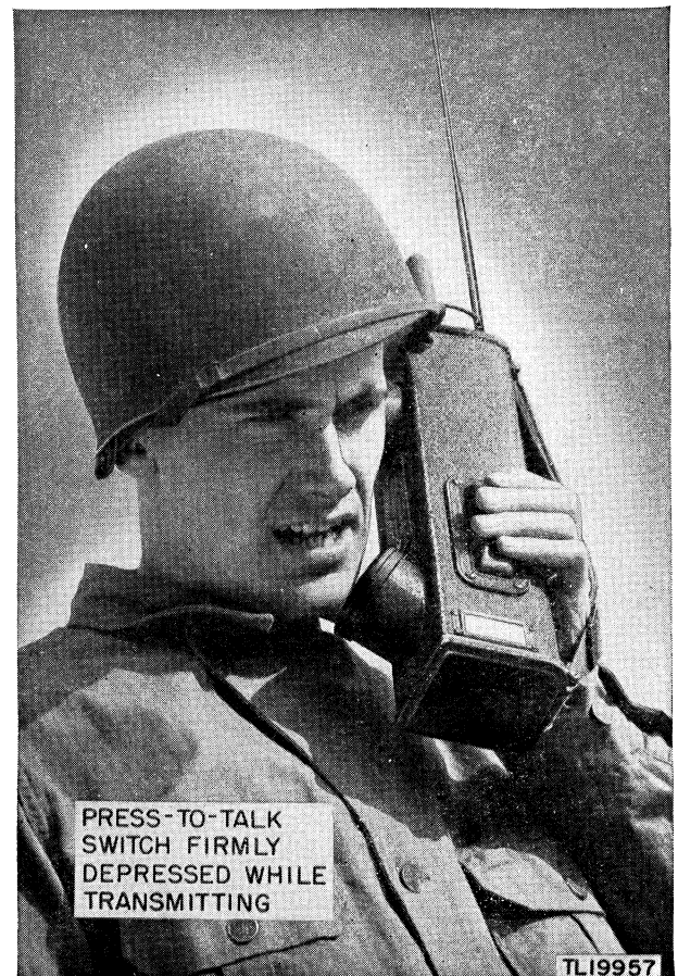
Figure 20. Radio Set SCR-536-(*), transmitting position.
